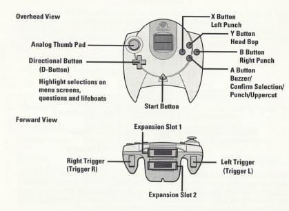
Never touch the Analog Thumb Pad or Triggers L/R while turning the Sega Dreamcast power ON. Doing so may disrupt the controller initialization procedure and result in malfunction. If the Analog Thumb Pad or Triggers L/R are accidentally moved while turning the Sega Dreamcast power ON, immediately turn the power OFF and then ON again making sure not to touch the controller.
